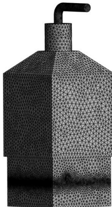
Gambar 2. Hasil meshing model boiler stoker
