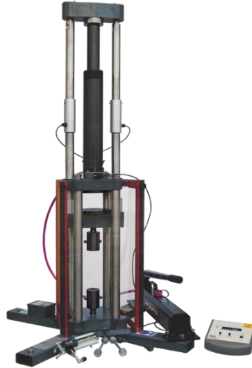
Gambar 1. Universal testing machine SM 1000
