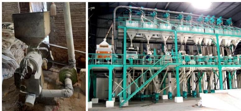
Gambar 1. Rice Milling Unit (Kiri) dan Rice Milling Plant (Kanan)
