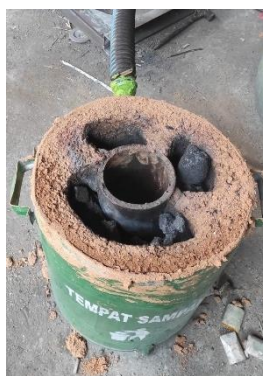
Gambar 3. Tungku Hot Dip Galvanizing
