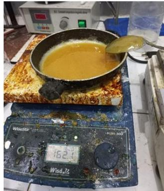
**Gambar 1.** Proses Pencampuran Gondorukem, Terpentin, *Plasticizer*, dan Katalis MEKPO
