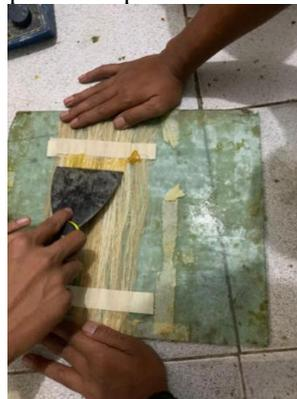
**Gambar 2.** Proses *Hand Lay-Up*
