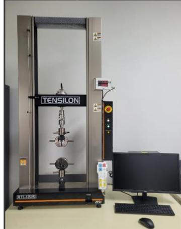
Gambar 6 *Universal Testing Machine* Tensilon
