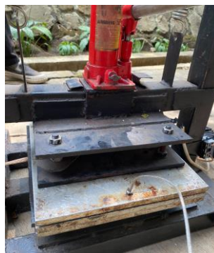
Gambar 4. Proses hot compression
