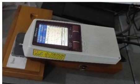
Gambar 7. Mitutoyo Surface Test SJ-210
