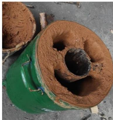
Gambar 3. Tungku Hot Dip Galvanizing
