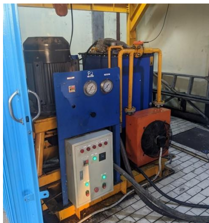
Gambar 1. Pompa Hydraulic Axial 250 LPS
