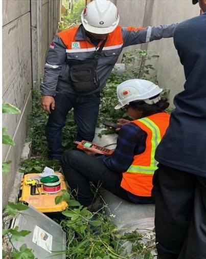
**Gambar 1.** Pengujian *Flowrate* Pompa *Hydraulic Axial 250 LPS*
