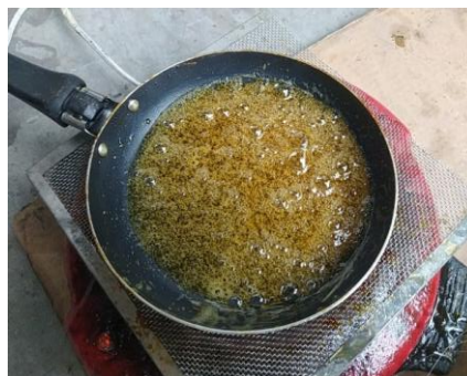
Gambar 3. Proses mencairkan campuran matriks gondorukem
