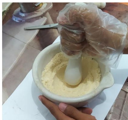
Gambar 2. Proses penghalusan gondorukem
