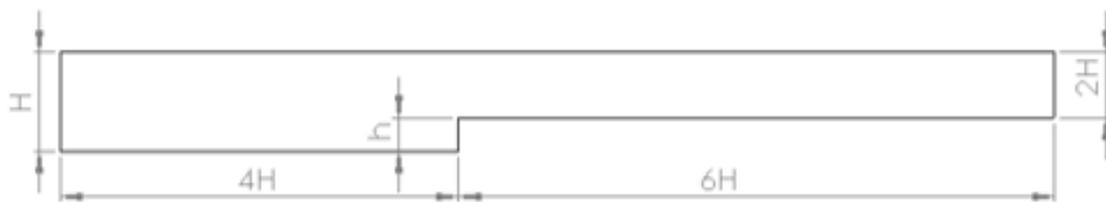
Gambar 1. Geometri model *forward-facing step*.
