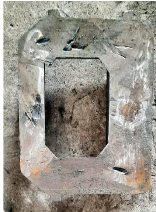
Gambar 19. Hasil Pengecoran Gating System 6 (Gambar Pribadi)
