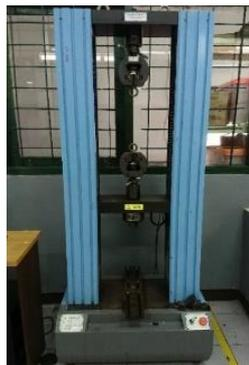
Gambar 9. *Universal Testing Machine* GD 1000-100
