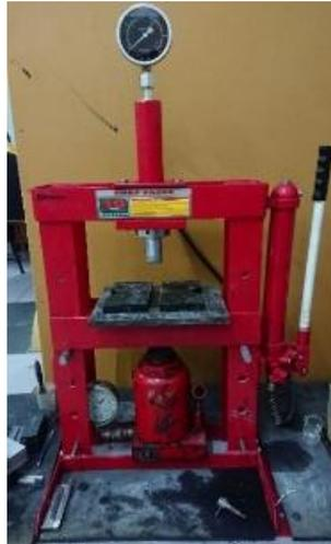
Gambar 4. *Hydraulic Press Machine*
