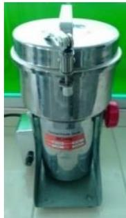
Gambar 1. Mesin *Electrical Powder Grider*
