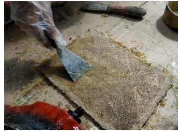
Gambar 5. Proses Hand Lay-Up
