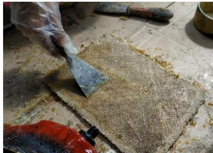
**Gambar 2.** Proses *Hand Lay-Up*
