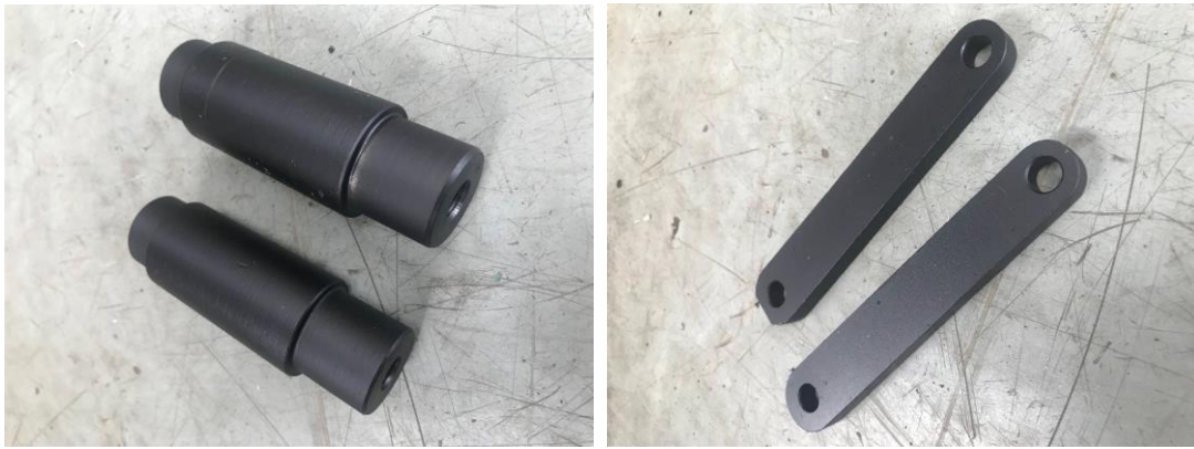
(a) (b) Gambar 25. Komponen (a) C bushing dan (b) rod to wheel support .
