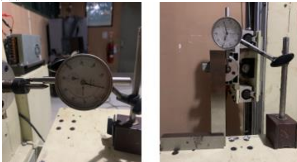
Gambar 6. Pengujian runs out of truth spindle .
