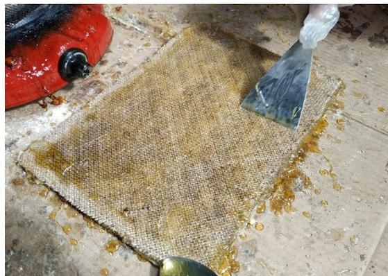
Gambar 2. Proses *Hand Lay-Up*
