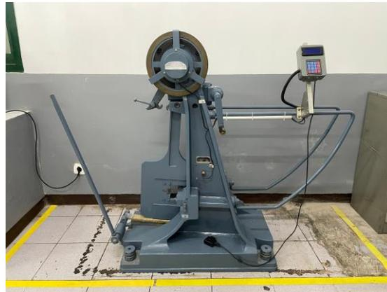
Gambar 3. *Impact Testing Machine*
