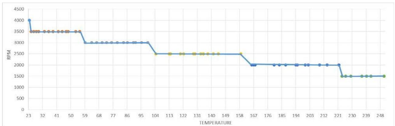
Gambar 7. Grafik Braking Cycle Kampas Rem OES.
