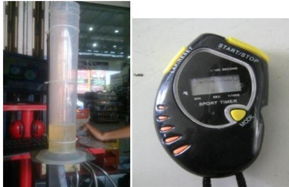
Gambar 6. (a) gelas ukur (b) *stopwatch*
