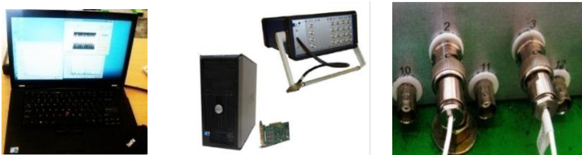
Gambar 7. (dari kiri) Laptop data akuisisi, DAQ (data acquisition systems), Kabel bayonet naur connector (BNC) dan connector [2]
