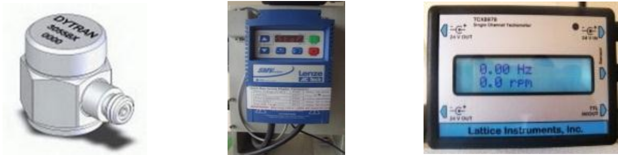
Gambar 6. (Dari kiri) Sensor accelerometer, Inverter speed control, Tachometer digital display [2]
