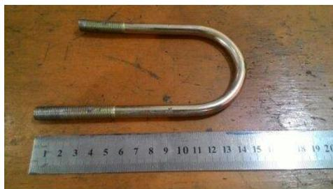
**Gambar 2.** *Clamp U* patah [1]
