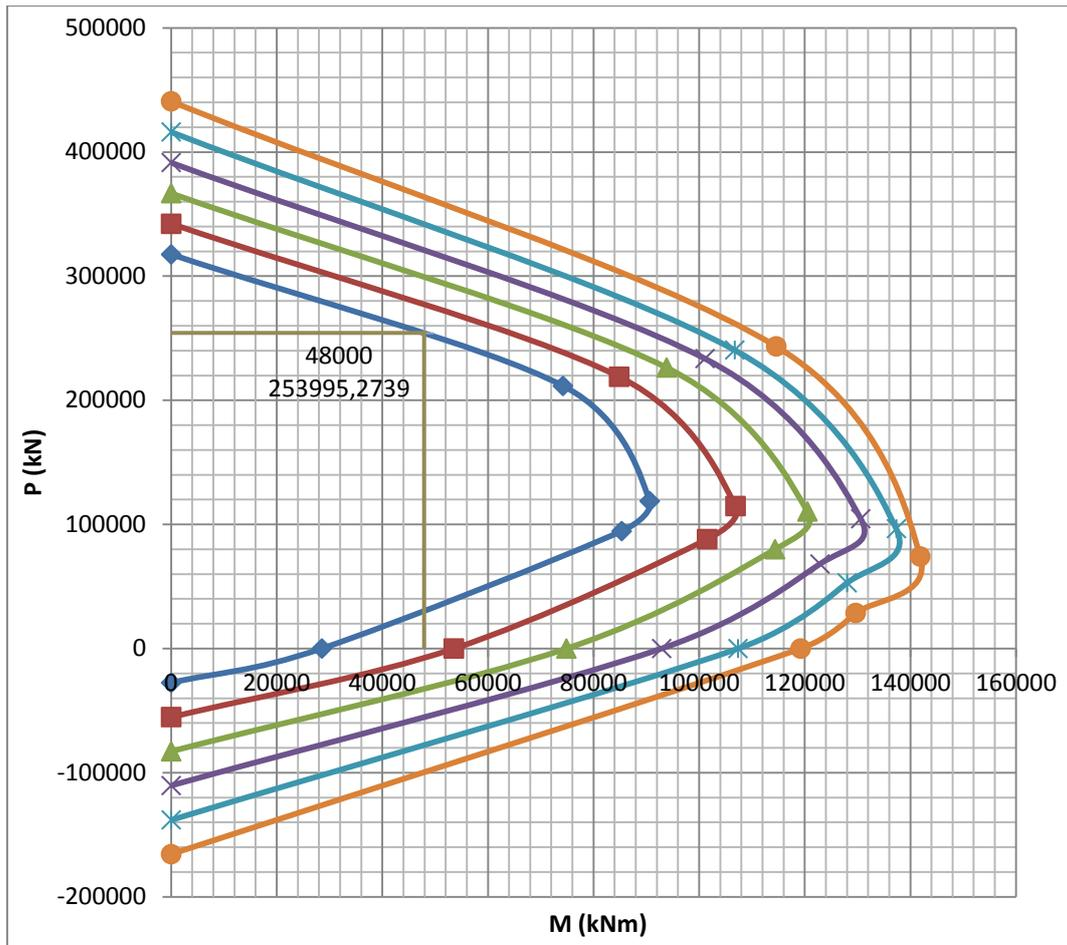
Gambar 10 Diagram Interaksi 1% – 6% M22
