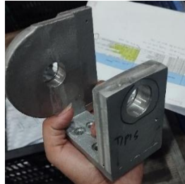
Gambar 4. 5 Gambar Defect Lubang Gear Box Terlalu Tipis
