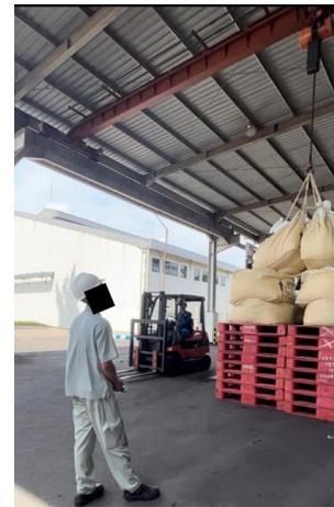
**Gambar 12** Pekerja 3 Pengoperasian Mesin *Hoist Crane*
