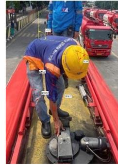
**Gambar 3.** Operator 3 Membuka *Upper manhole*
