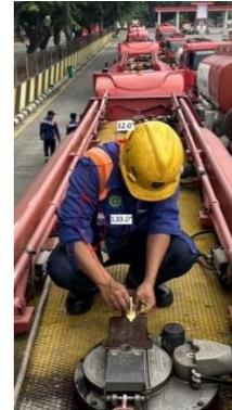
**Gambar 12.** Operator 5 Memasang Segel Upper manhole
