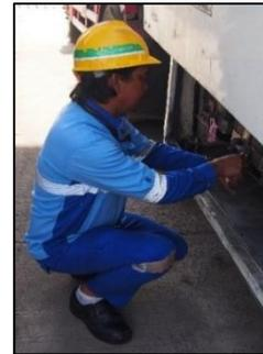
**Gambar 7.** Operator 7 Memasang Segel *Manhole Bottom*
