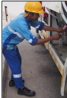
**Gambar 6.** Operator 6 Memasang Segel *Manhole Bottom*
