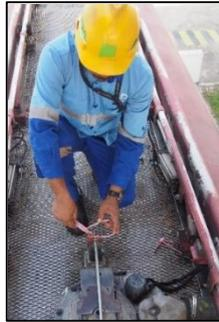
**Gambar 15.** Operator 7 Memasang Segel *Manhole Upper*
