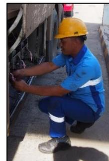
**Gambar 8.** Operator 8 Memasang Segel *Manhole Bottom*
