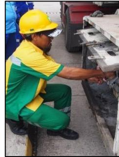
**Gambar 4.** Operator 4 Memasang Segel *Manhole Bottom*
