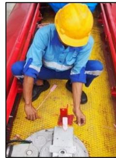
**Gambar 14.** Operator 6 Memasang Segel *Manhole Upper*
