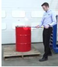
**Gambar 3. Drum Lever Bar**
