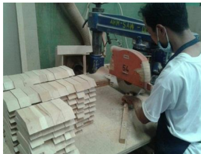
Gambar 9 Proses Operasi Mesin Arm Saw
