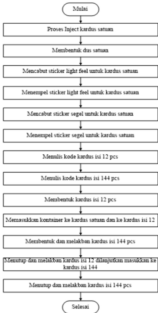
Gambar 1 Tahapan proses *packaging Lipstick Long Lasting*
