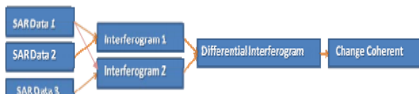
Gambar II. 2. Alur pengolahan SAR metode three-pass (ESA, 2007)
