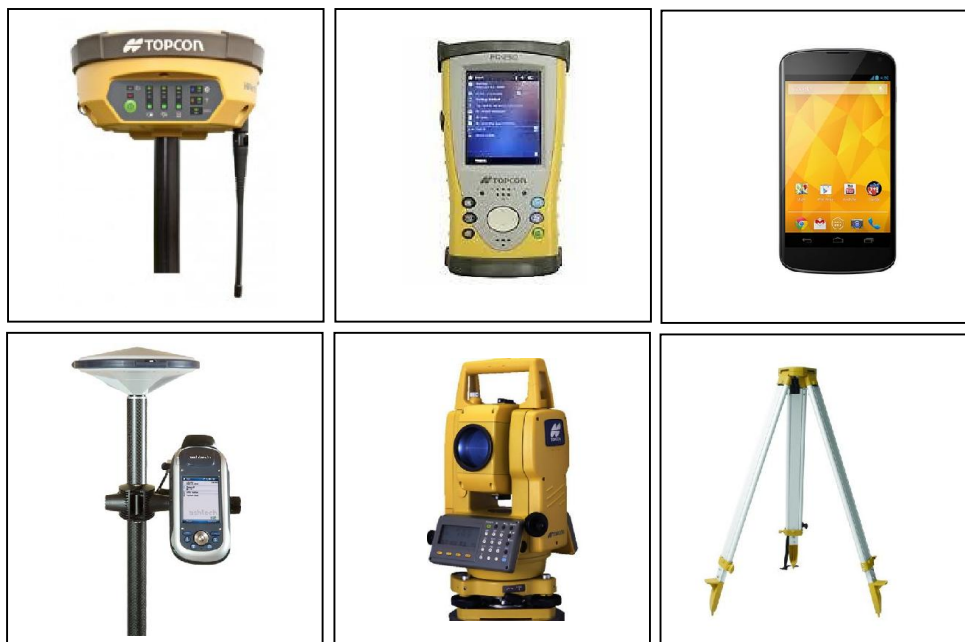
Gambar 3.2 Receiver Topcon Hiper II, Controller FC 250, Handphone LG-E960, Receiver PM-200, Total Station GTS 235 dan Statip
