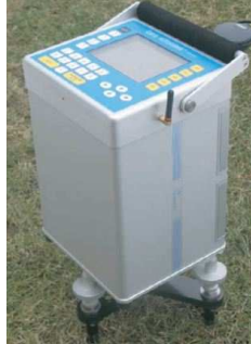
Gambar 2. Gravimeter Scintrex CG 5 [Scintrex Brochure]
