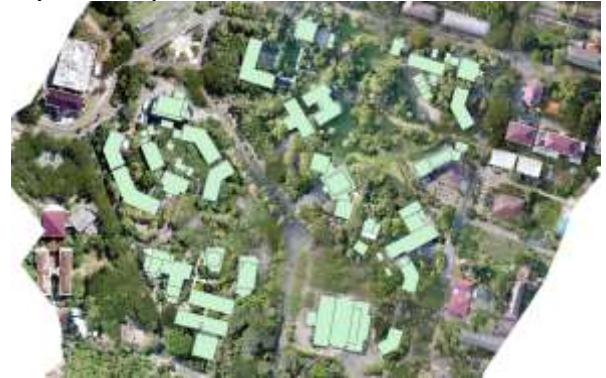
Gambar 10. Shapefile footprint bangunan
