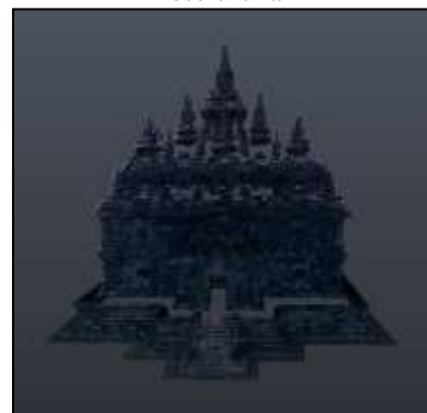
Gambar IV-4 Hasil Point Cloud TLS Model Terfilter
