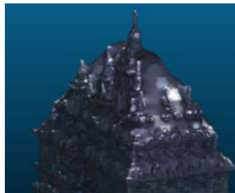
Gambar IV-6 Bagian Atas Candi Hasil Proses Poisson Surface Reconstruction
