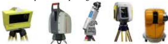
Gambar 2 Contoh alat Terrestrial Laser Scanner (Quintero dkk, 2008)
